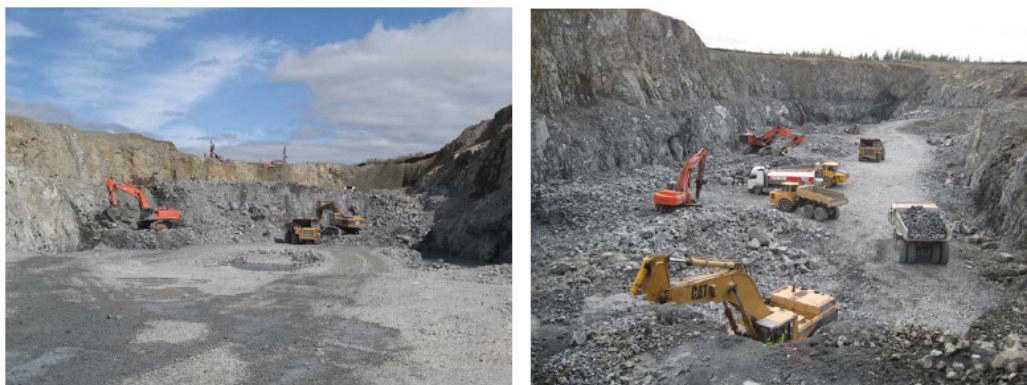
Figure 61: excavation of good quality vulcanite rock for roads and tailing dams from the western side of the Suurikuusikko pit between September 2006 and July 2007
